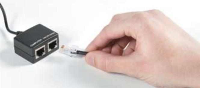
4. Plug one end of the other Ethernet cable into the Ethernet jack marked **COMPUTER** on the power supply.
