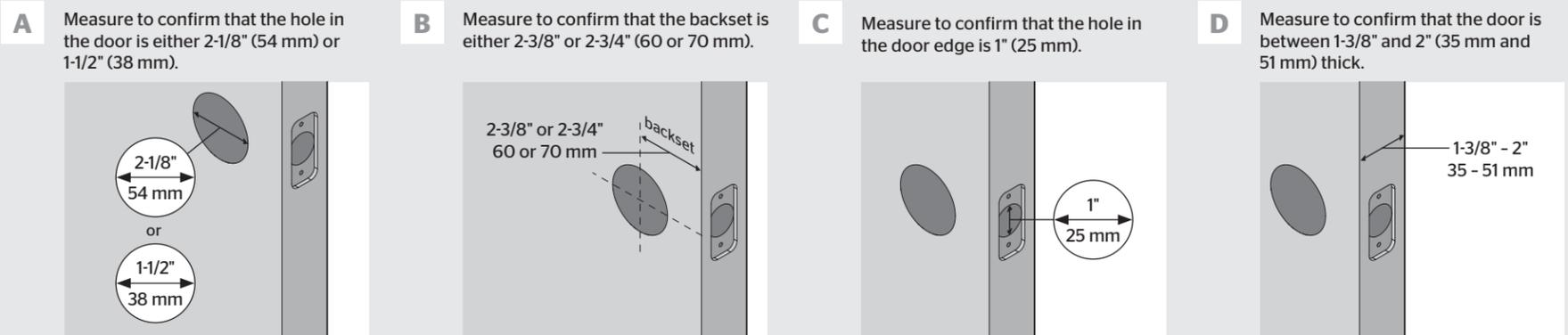
Note: Additional door preparation may be required for doors with 1-1/2" (38 mm) holes. Consult the deadbolt drilling instructions at [www.weiserlock.com/doorprep](http://www.weiserlock.com/doorprep).
