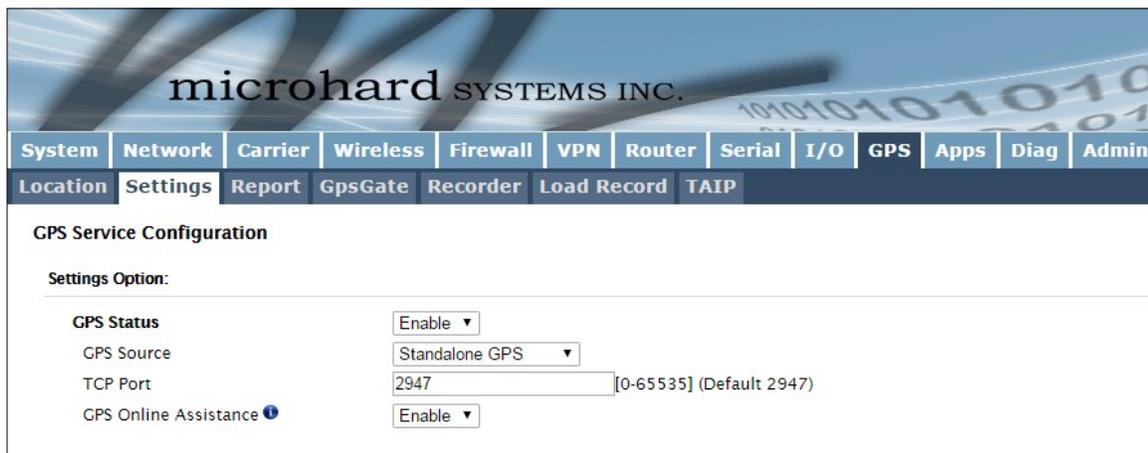
The screenshot shows the 'GPS Service Configuration' page in the BulletPlus web interface. The navigation menu includes System, Network, Carrier, Wireless, Firewall, VPN, Router, Serial, I/O, GPS, Apps, Diag, and Admin. The sub-menu includes Location, Settings, Report, GpsGate, Recorder, Load Record, and TAIP. The 'Settings Option' section contains the following fields:
